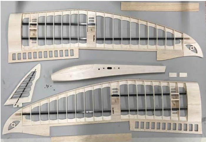
The obligatory sanded framework photo before covering.
