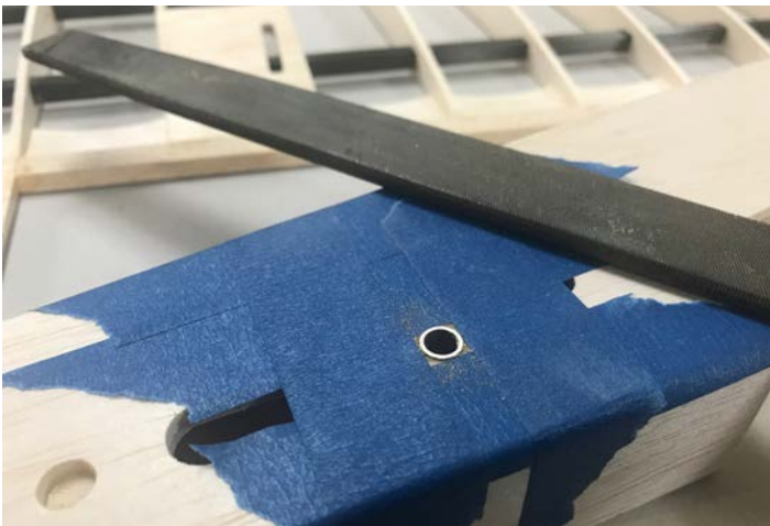
Tape around the brass insert tubes to file down...
